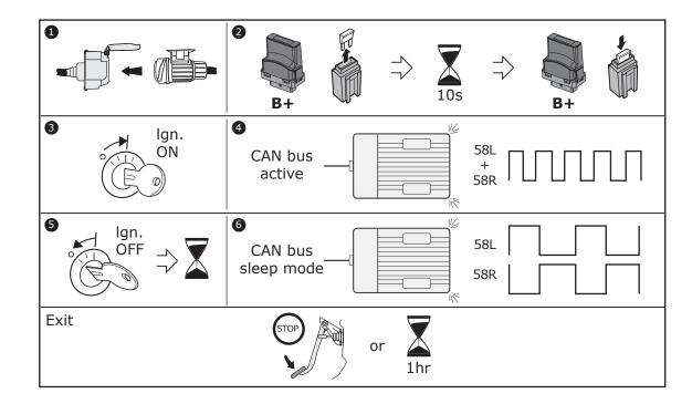
The faultless connection of the trailer module to the vehicle-side CAN-bus can be checked quick and easy with the ECS CAN-check:
