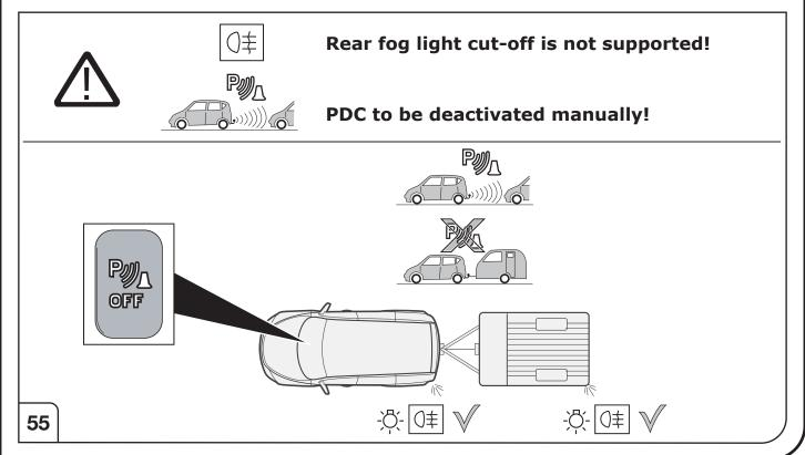
The following light functions for the trailer are not **supported** by all towing vehicles **with DRL circuit:**
