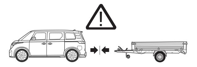
This kit does not support any of the assistance systems of the vehicle. Vehicle assistance systems may have to be deactivated manually when towing a trailer!
